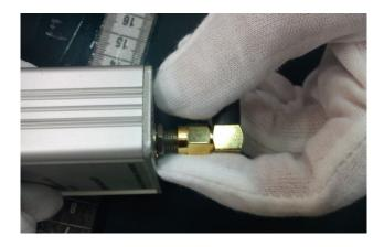
2) Use torque wrench which has 0.9 Nm torque limit to tighten it.
