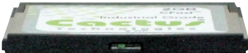
Figure 2-2. Type I CFast Card with Write Protect switch
